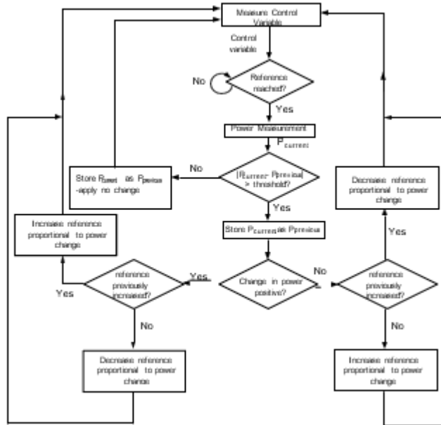
Figure 12: General MPPT Flow Chart for wind and PV
